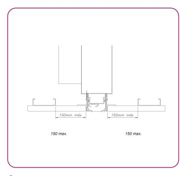
**6.-** Push the diffuser lightly downwards and screw the sheets to the fixing profile.
