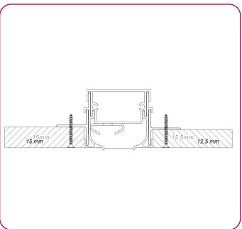
**5.-** Cut the sheet of plasterboard in two and place the sheets against the diffuser and its fixing/line formation profile.
