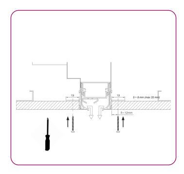
**4.-** When installing in lines, the fixing profile should be extended approximately 60 mm out from the end of the diffuser.
