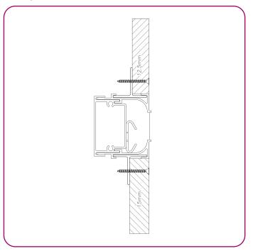
**4.-** Gently support the diffuser and screw plasterboard to the mounting frame.
