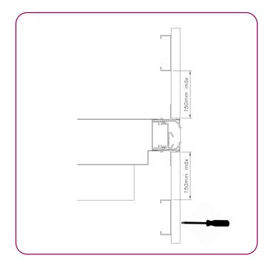
**5.-** Tape the lower surface of the diffuser for subsequent filling with a thick paste. Finish with a fine paste.
