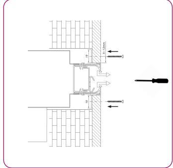
**6.-** Tape the lower surface of the diffuser for subsequent filling with a thick paste. Finish with a fine paste.
