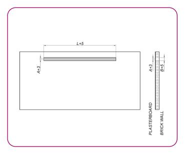
**3.-** Support the diffuser on plasterboard as shown in the figure. If a plenum is used, fix using threaded drop rods and lugs at the rear of the plenum.
