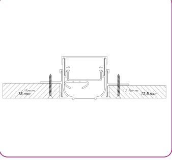
**4.-** It is recommended that the secondary structure be placed at a maximum distance of 150 mm from the outside edge of the diffuser.
