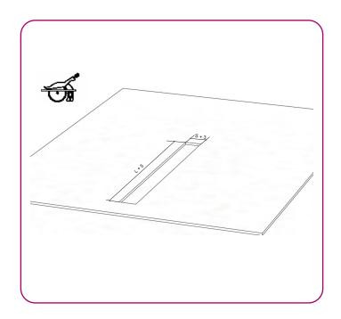
**2-** Turn the diffuser and raise it through the hole. Once through the plasterboard, turn back to horizontal and lower it so that it rests on the plasterboard.
