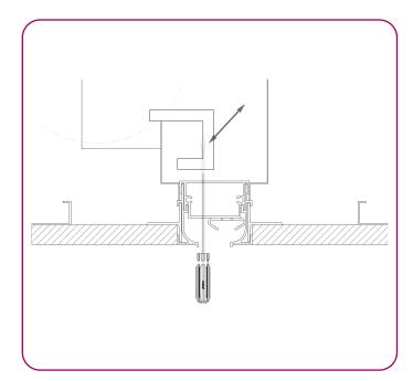
**13.-** Replace the plugs in the valve regulating holes.
