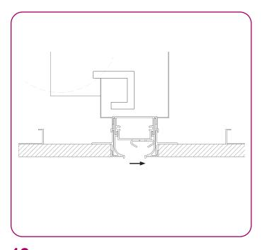
**12.-** Insert a screwdriver through the hole in the blade and turn the regulating rod until the valve is set in the desired position.
